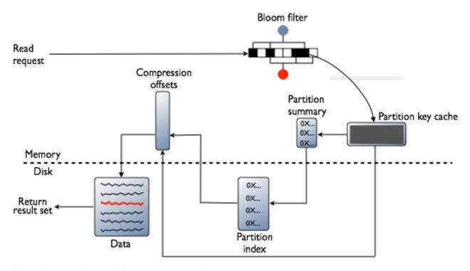
Figure: Row cache and Key cache request flow
